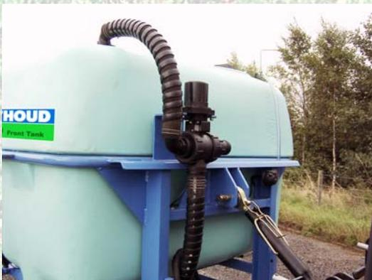
Electrically operated transfer valve to allow controlled transfer while pump is in the agitation mode. Controlled by a switch in the cab.
